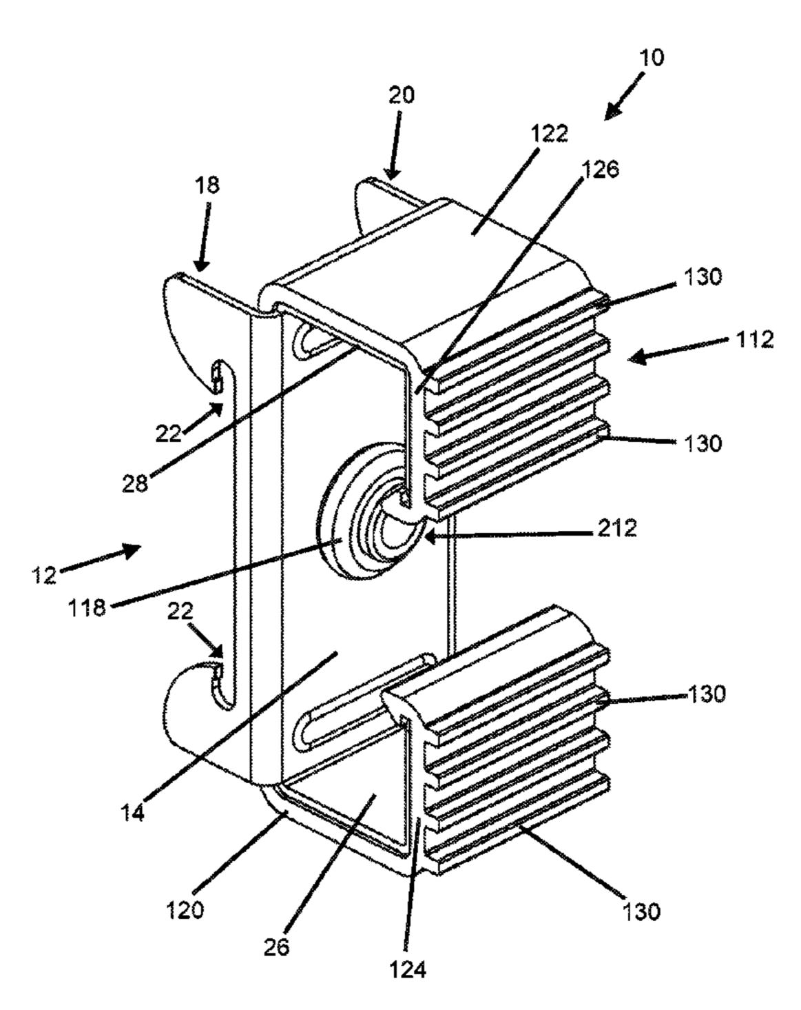
extending transversely from each of the at least one leg portion, wherein in use, when the body portion is attached relative to the support structure, each foot portion is proximal to the support structure and each of the at least one connection portion is distal to the support structure.
