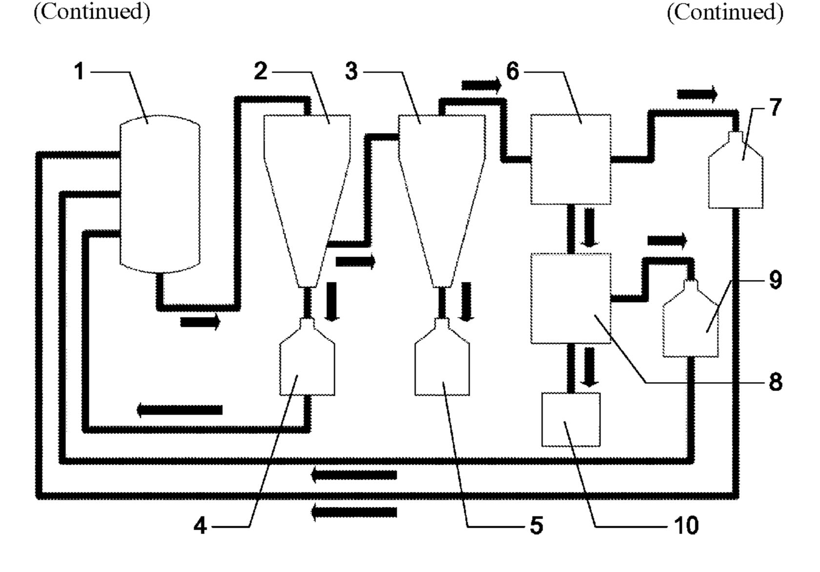
having an enclosed vessel for receiving a solvent or surfactant mixture with dispersed particles of a crystalline graphitic material. The reactor can be arranged for: submitting the mixture in the enclosed vessel to a cavitation force such that cavitation bubbles are present and, simultaneously in the same enclosed vessel, submitting the mixture to high shear agitation.
