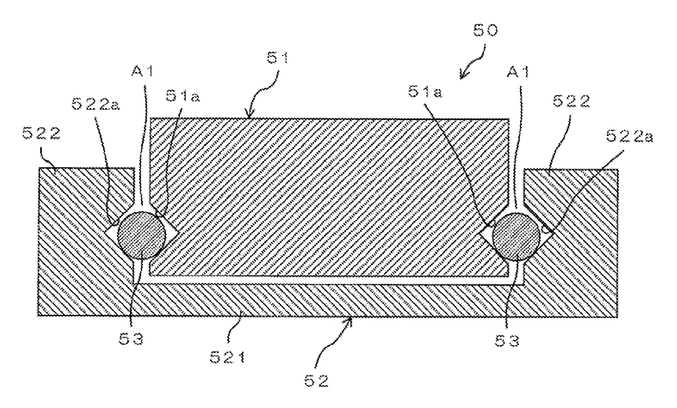
Accordingly, when the movable mirror and the movable portion are slid, it is possible to suppress rattling of the movable portion and the holding portion while leaving a fine gap between the movable portion, the holding portion, and each rolling element. This makes it possible to easily control the moving speeds of the movable mirror and the movable portion and to suppress rattling of the movable mirror and the movable portion.
