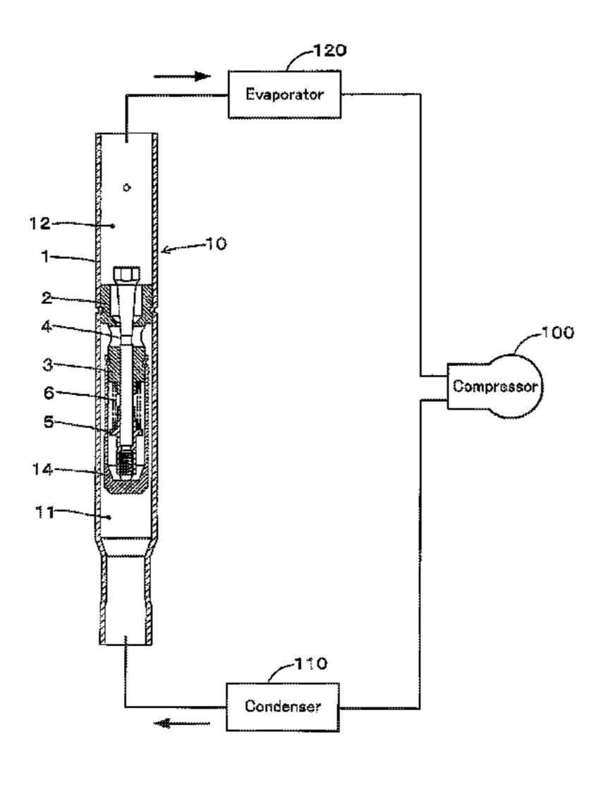
main body case functions as a main body path for delivering a refrigerant from the primary chamber to the valve port.
