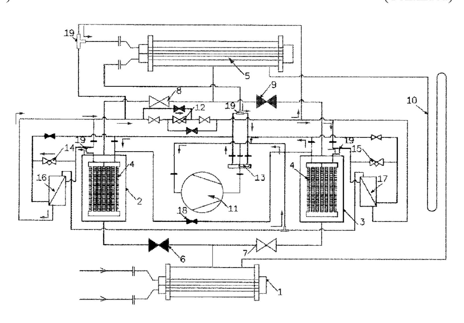
process and/or condensation process of the adsorption cycle is pumped to the desorption process. Thus, this new hybrid combined cycle becomes a partially or fully electricity driven heat pump cycle.
