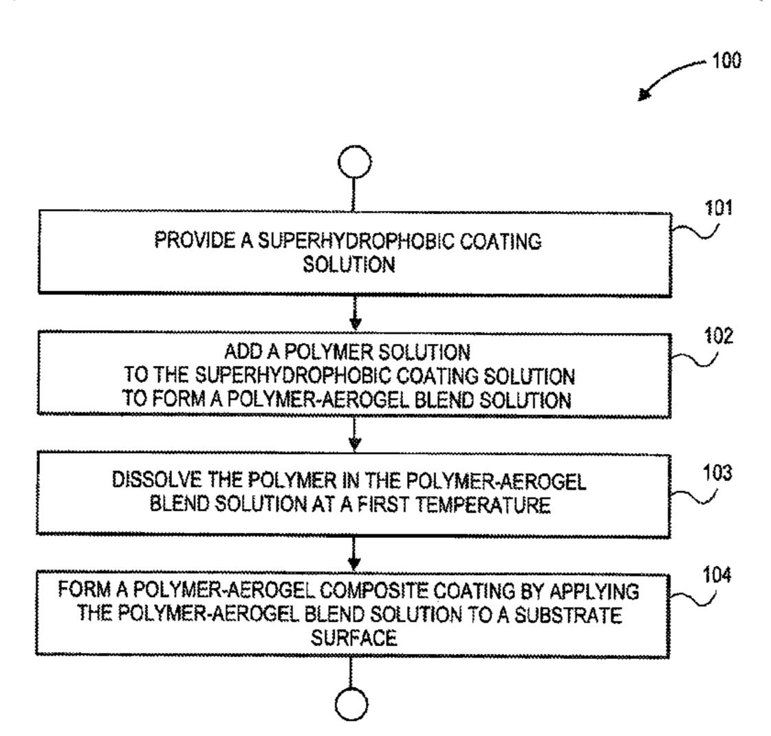
posite coating can include a polymer and an ultra high water content catalyzed polysilicate aerogel, the polysilicate aerogel including a three dimensional network of silica particles having surface functional groups derivatized with a silylating agent and a plurality of pores.
