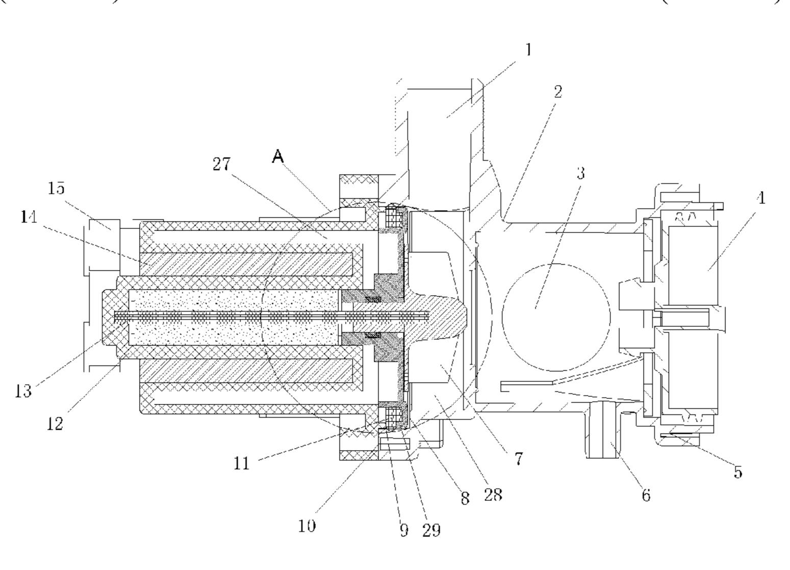
plate, enters the motor cavity, and is connected with the pump shaft in the motor cavity.
