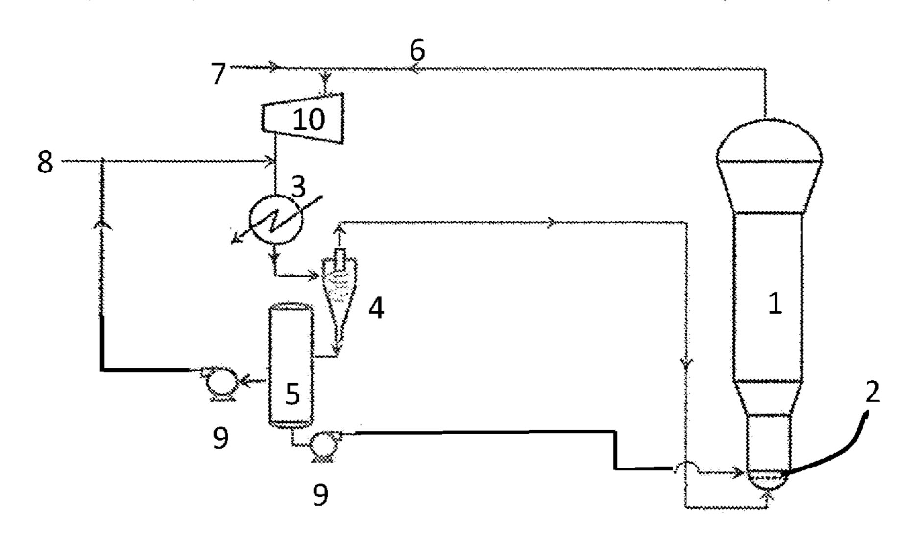
a distribution plate (e) introducing the liquid phase to a settling tank to separate liquid from fines that settle down in the settling tank (f) introducing liquid from the settling tank up stream of the cooling unit.
