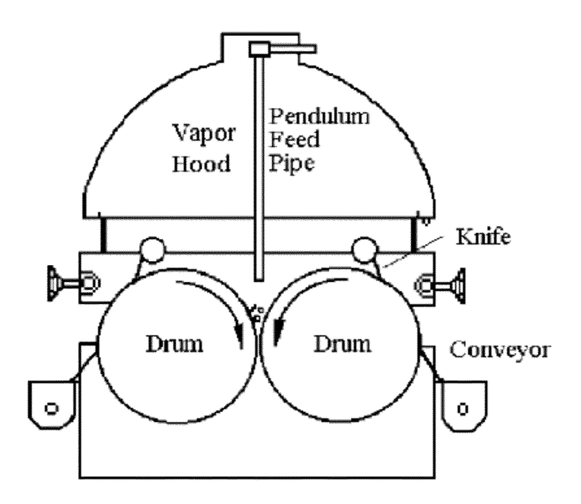
Schematic representation of double drum dryer
