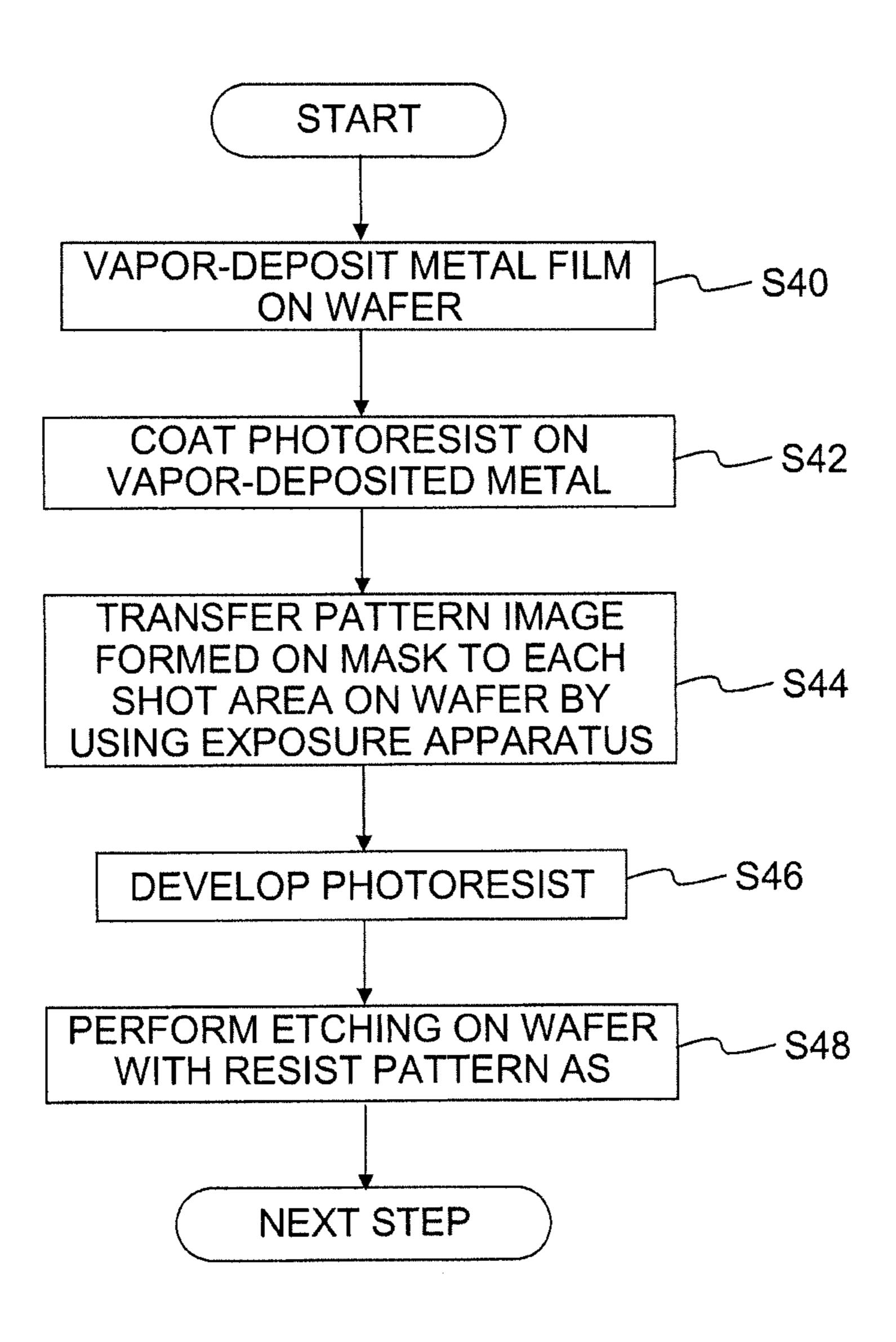
LIGHT SOURCE APPARATUS, OPTICAL APPARATUS, EXPOSURE APPARATUS, DEVICE MANUFACTURING METHOD, ILLUMINATING METHOD, EXPOSURE METHOD, AND METHOD FOR MANUFACTURING OPTICAL APPARATUS
