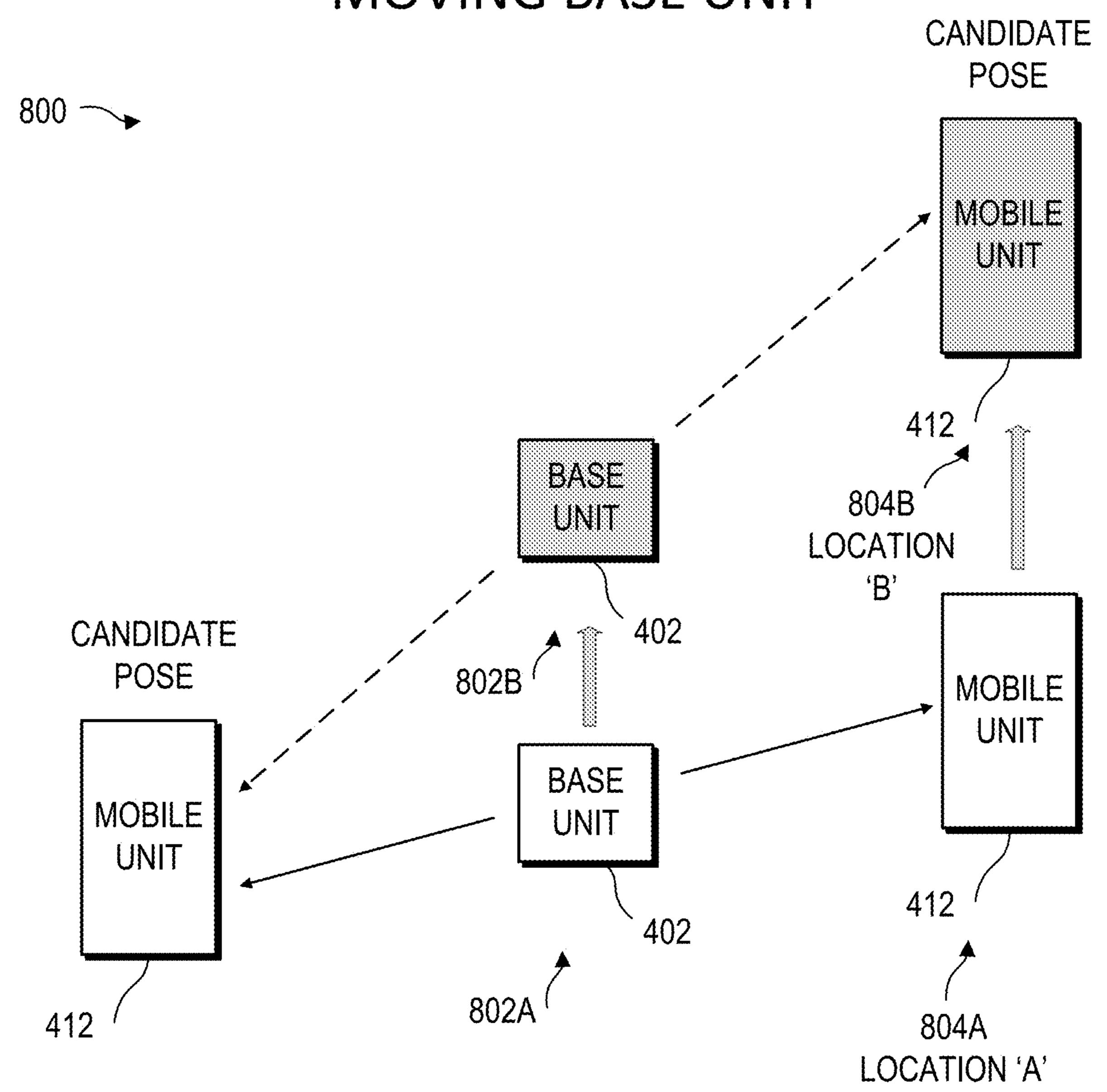
WHEN BASE MOVES LATERALLY RELATIVE TO A STATIONARY MOBILE UNIT, THE WORLD FRAME POSITION OF THE ACTUAL POSE DOES NOT CHANGE
