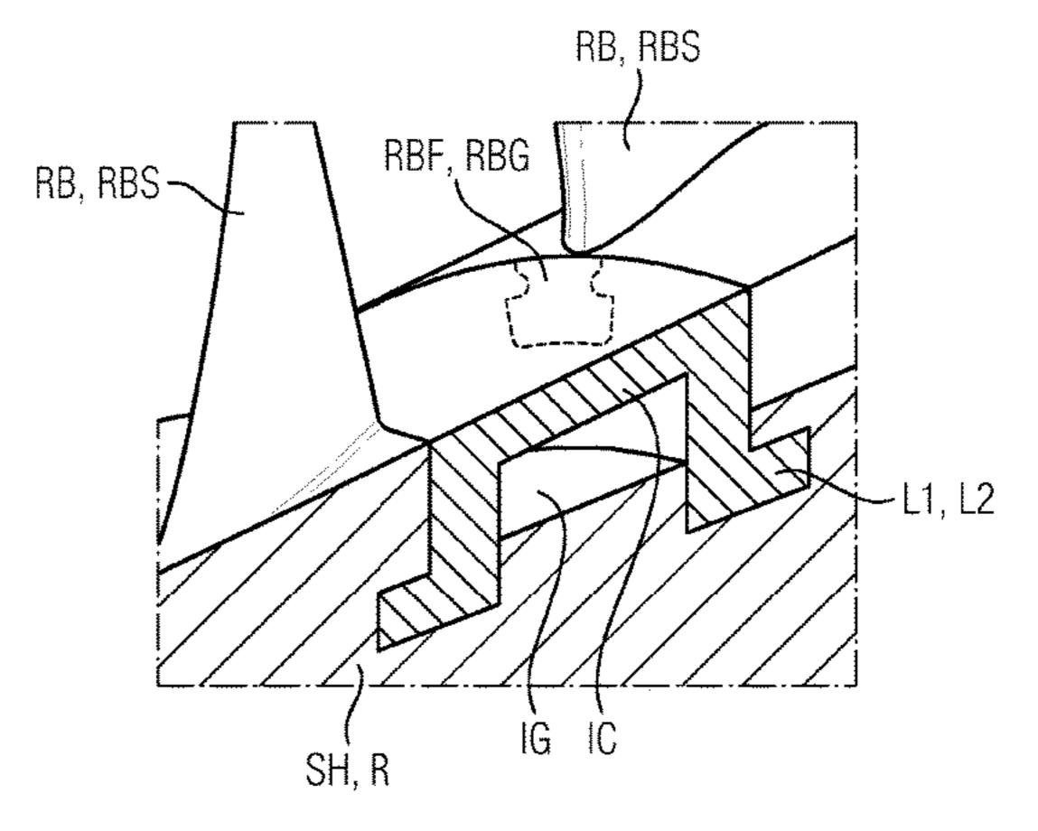
wherein the interspace cover is designed segmented into interspace cover segments in the circumferential direction.
