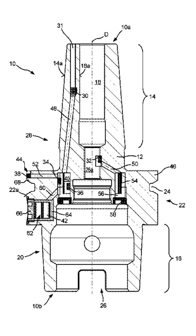
energy supply apparatus (42) that is connected to the signal transfer apparatus (38) and to the electrical circuit (40). According to the present invention the tool holder (10) comprises a tool holder main body (12) that comprises both the tool segment (14) and the coupling segment (16), at least one component from among the sensor (30, 32, 34, 36), electrical circuit (40), and energy supply apparatus (42) being received in a recess (56, 62) in the interior of the tool holder main body (12).
