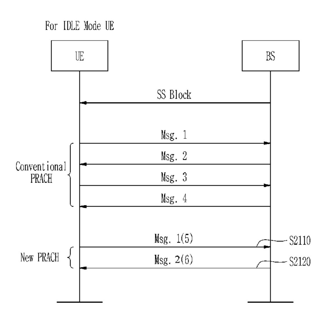
used to transmit the message 1; and transmitting the message 2 by using the optimal transmission beam.
