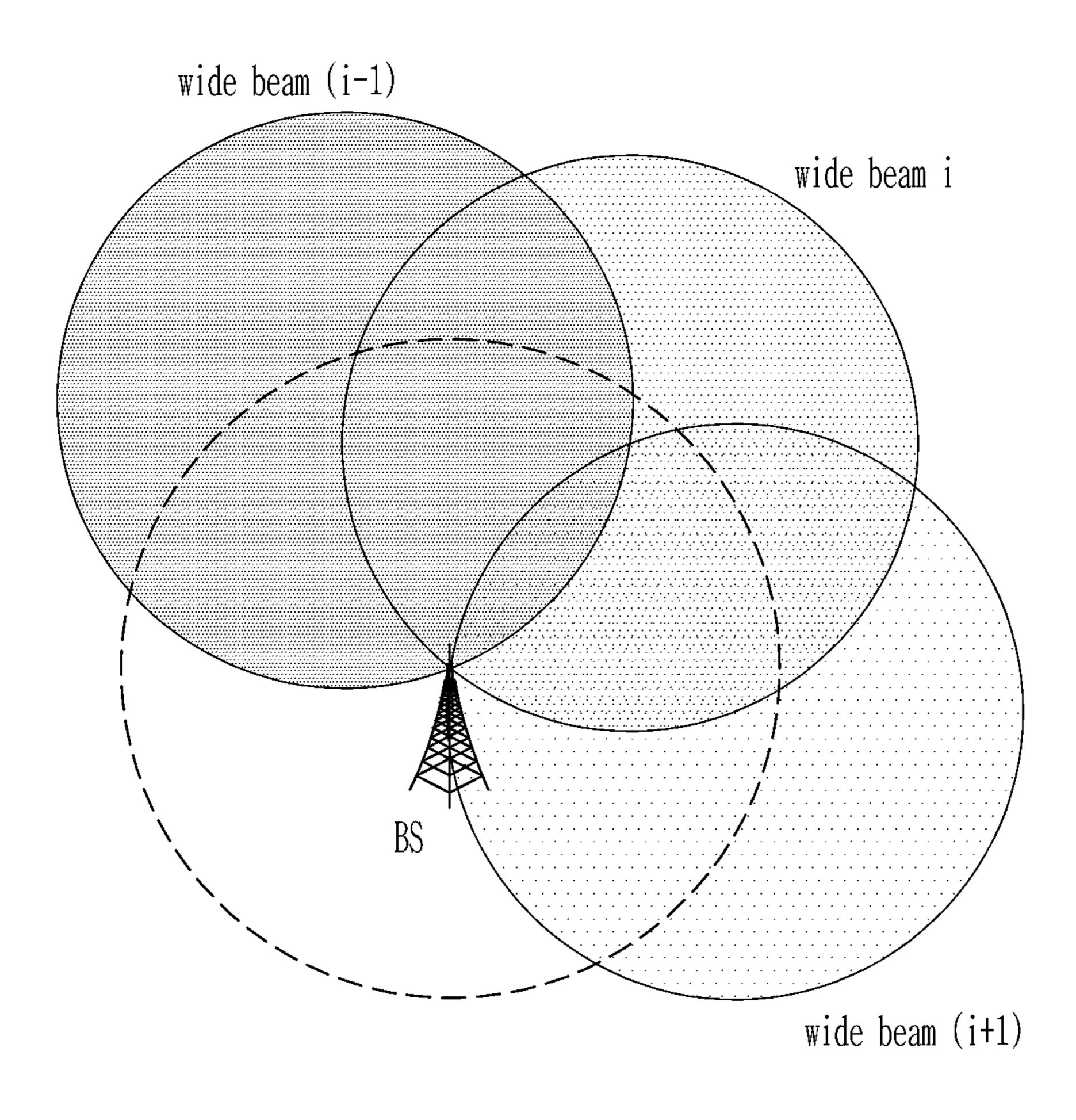
preamble RA preambl RA preamble Wide beam directions for RA procedure Original narrow beam directions narrow
