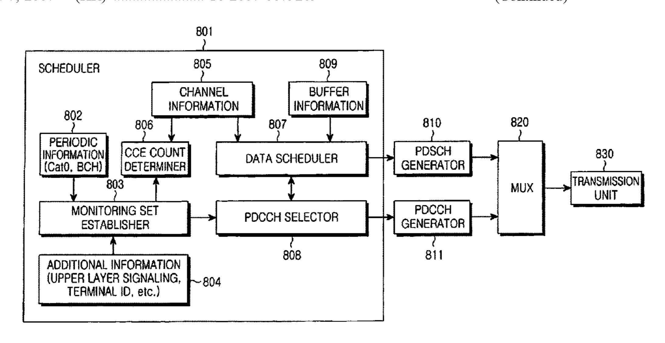
IDentifier (ID) of the terminal and the information associated with the number of CCEs, wherein each control channel candidate includes one, two, four, or eight CCEs; selecting at least one control channel candidate from among the set of control channel candidates; and transmitting the control information to the terminal via the selected at least one control channel candidate.
