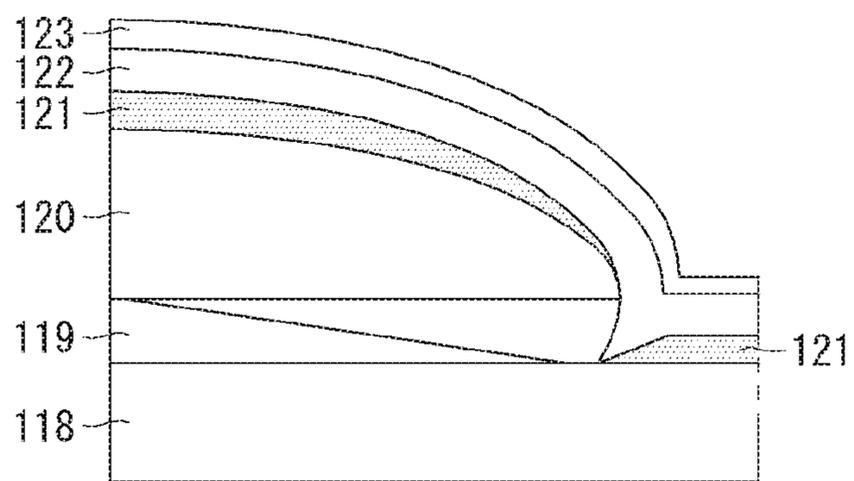
OLED fills the void to prevent cathode/PXL short-circuit
