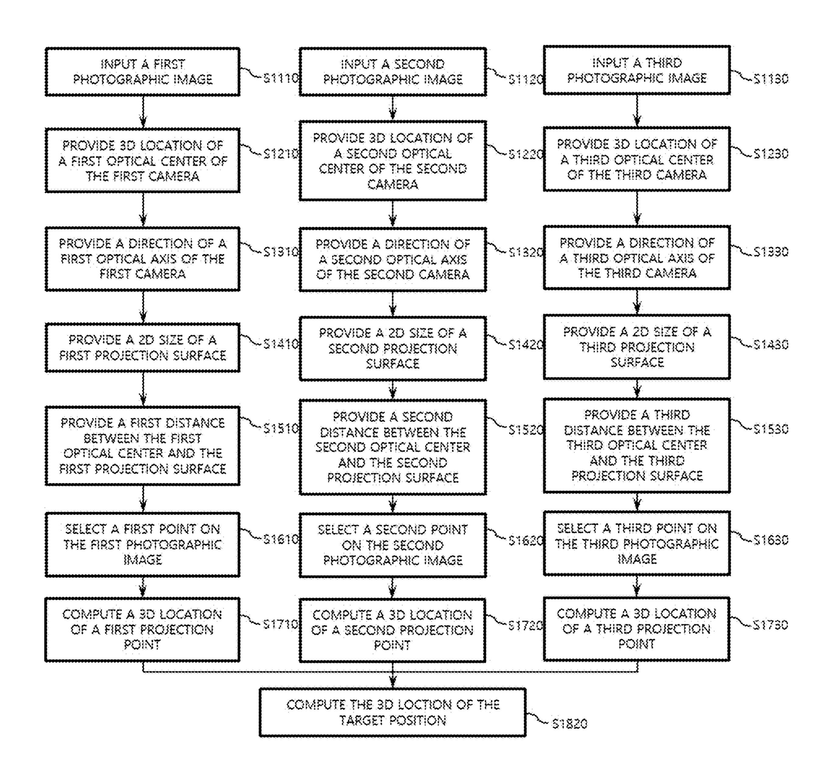
3 DIMENSIONAL COORDINATES CALCULATING APPARATUS, 3 DIMENSIONAL COORDINATES CALCULATING METHOD, 3 DIMENSIONAL DISTANCE MEASURING APPARATUS AND 3 DIMENSIONAL DISTANCE MEASURING METHOD USING IMAGES
