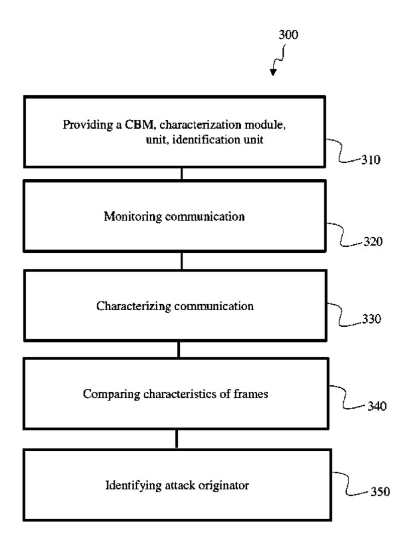
comparator, configured to identify at least one ECU originating an attack on the CAN bus.
