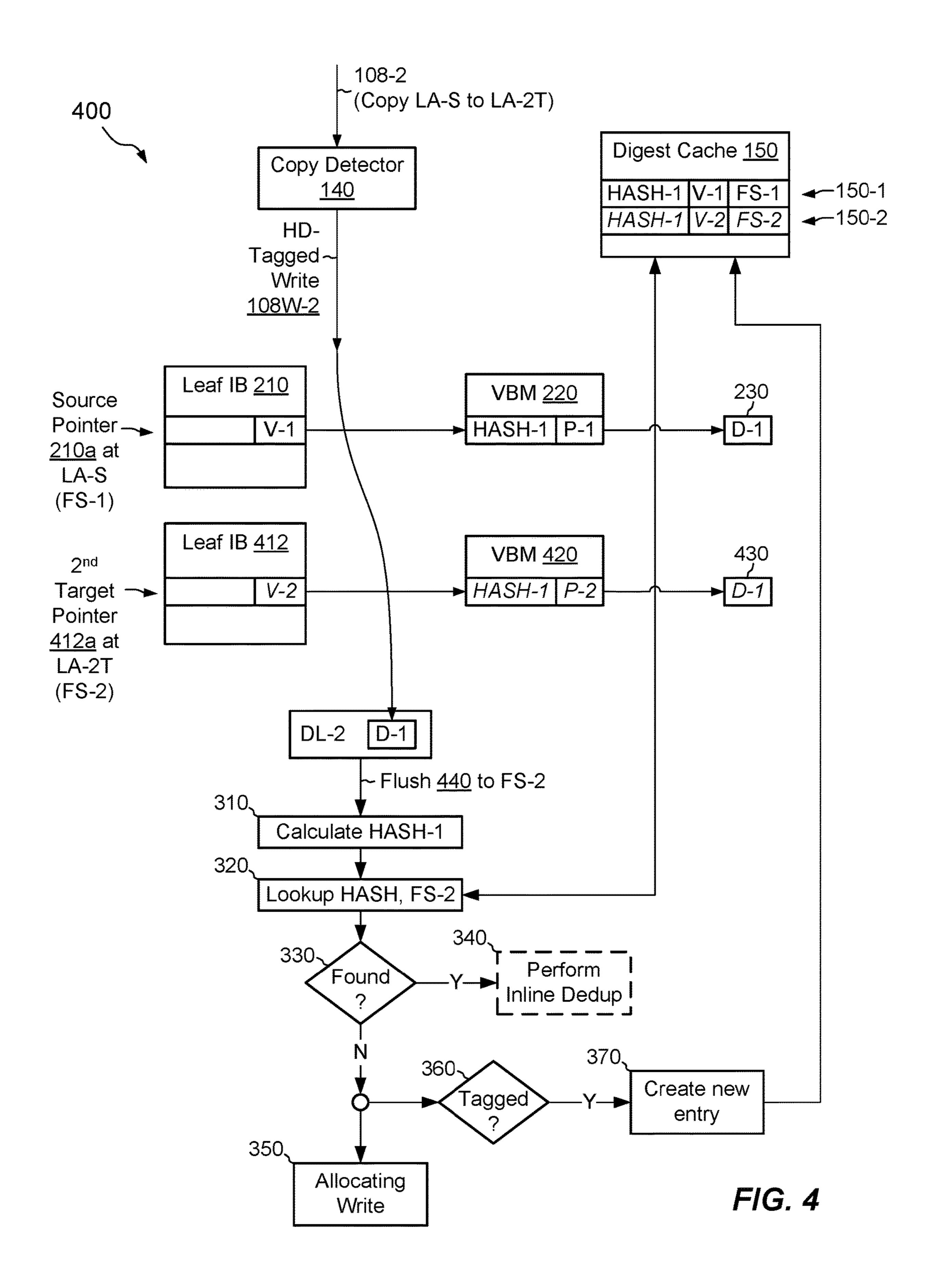
Receive a copy request that specifies copying of a set of data from a source logical address to a target logical address, the data storage system providing a source pointer for the source logical address and a target pointer for the target logical address, the source pointer having a value that points to the set of data
