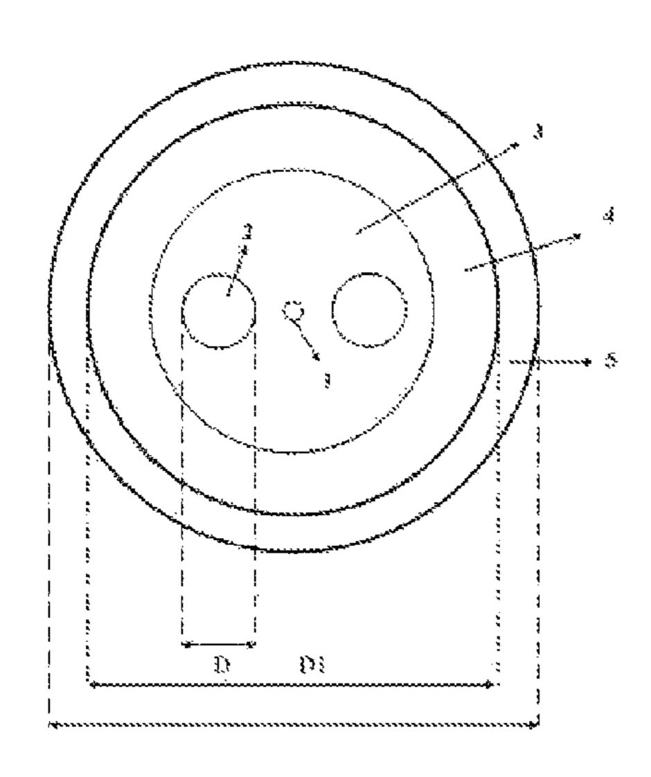
layer with a gradient refractive index. By providing the transition layer with the gradient refractive index at the edge of the outer side of the stress layer, the pressure stress at the edge of the stress layer is decomposed and released, so as to avoid cracks at the edge of the polished stress layer on the end of the optical fiber, and thus optimizes the performance of the polarization-maintaining optical fiber by decreasing the room temperature polishing cracking rate.
