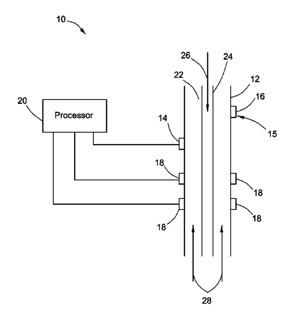
receive the first responsive signal and the second responsive signal, select one responsive signal according to a relationship of the first responsive signal and noise thereof and a relationship of the second responsive signal and noise thereof, and determine a flow rate of a flow medium according to the selected responsive signal. A method for measuring the flow rate of the fluid medium is also provided.
