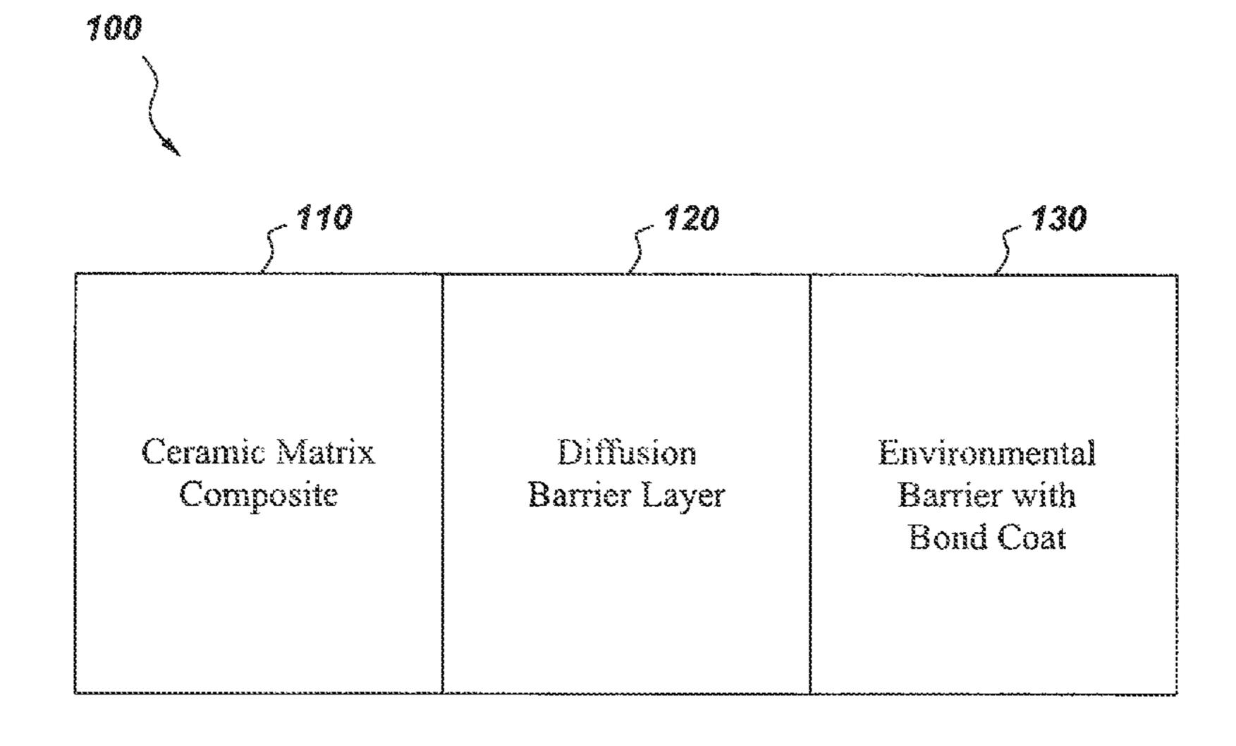
substrate to the bond coat of the environmental barrier coating system.
