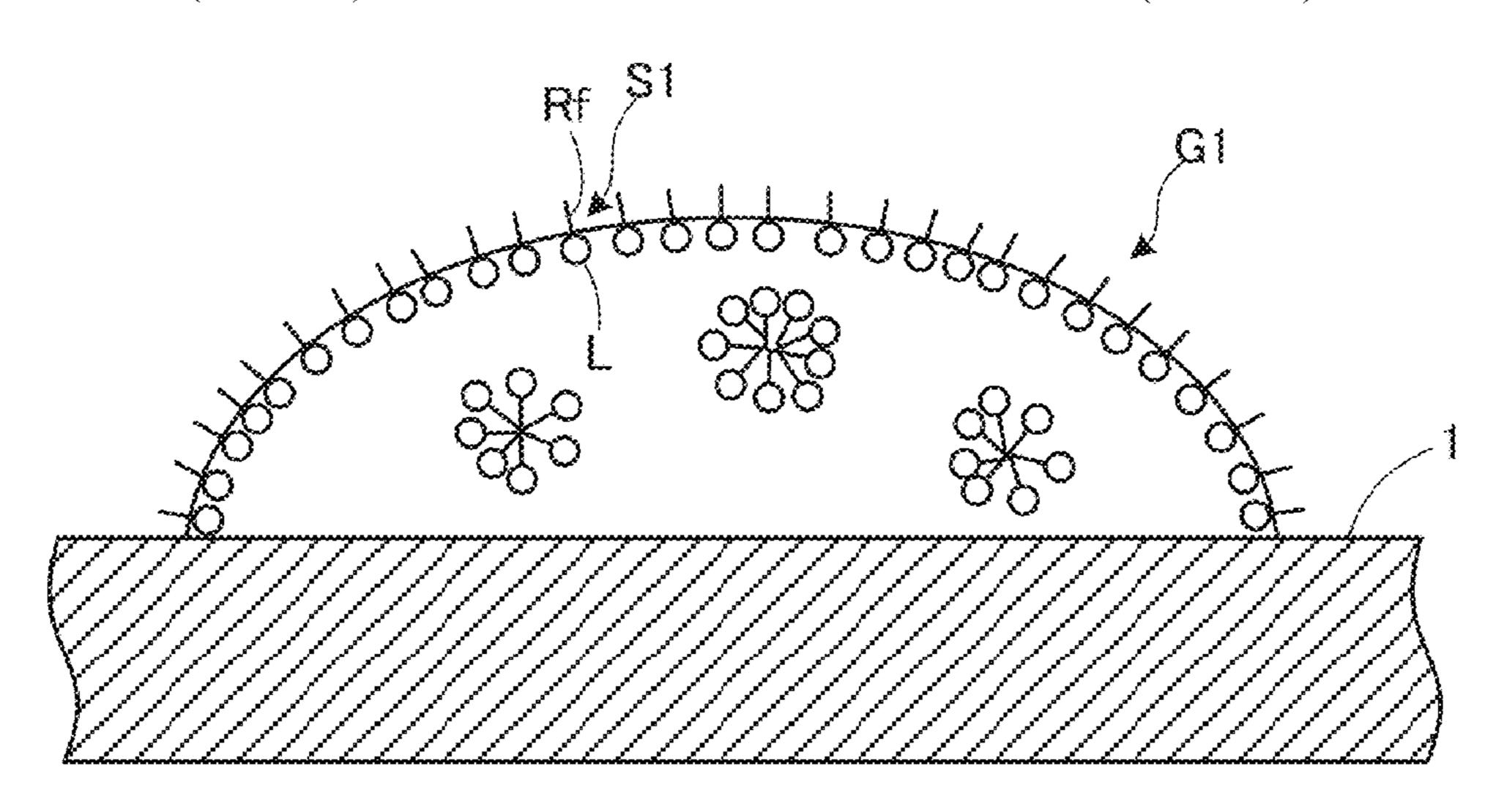
roalkyl group containing compound (S) having a perfluoroalkyl group or a fluoropolyether containing compound. As a result, foreign substance removing effects can be enhanced, and the lubricating properties can be improved as compared to the conventional lubricant compositions.
