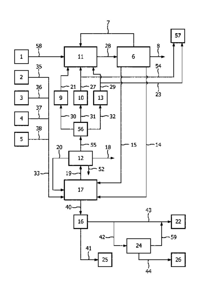
separating the stream thus hydrocracked in said hydrocracking unit into a high content aromatics stream and a gaseous stream comprising C2-C4 paraffins, hydrogen and methane,
