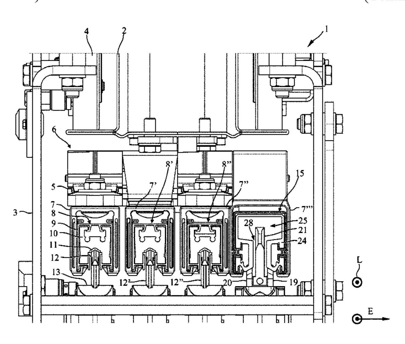
ductor rail, with at least one conductor strand extending in the longitudinal direction with an electrically conducting conductor profile for contacting a sliding contact of the load and with at least one data transmission device extending in the longitudinal direction.
