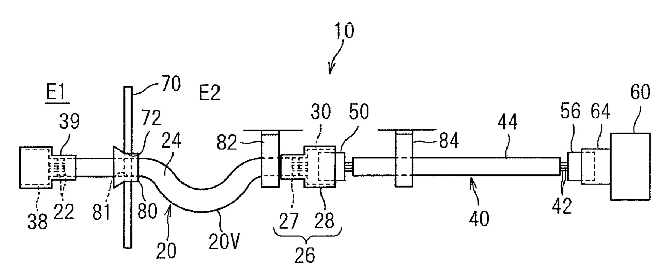
inter-wire water shut-off property; and a non-water shut-off cable being connected to the water shut-off cable in the exterior area, and being connectable to the connection target component.
