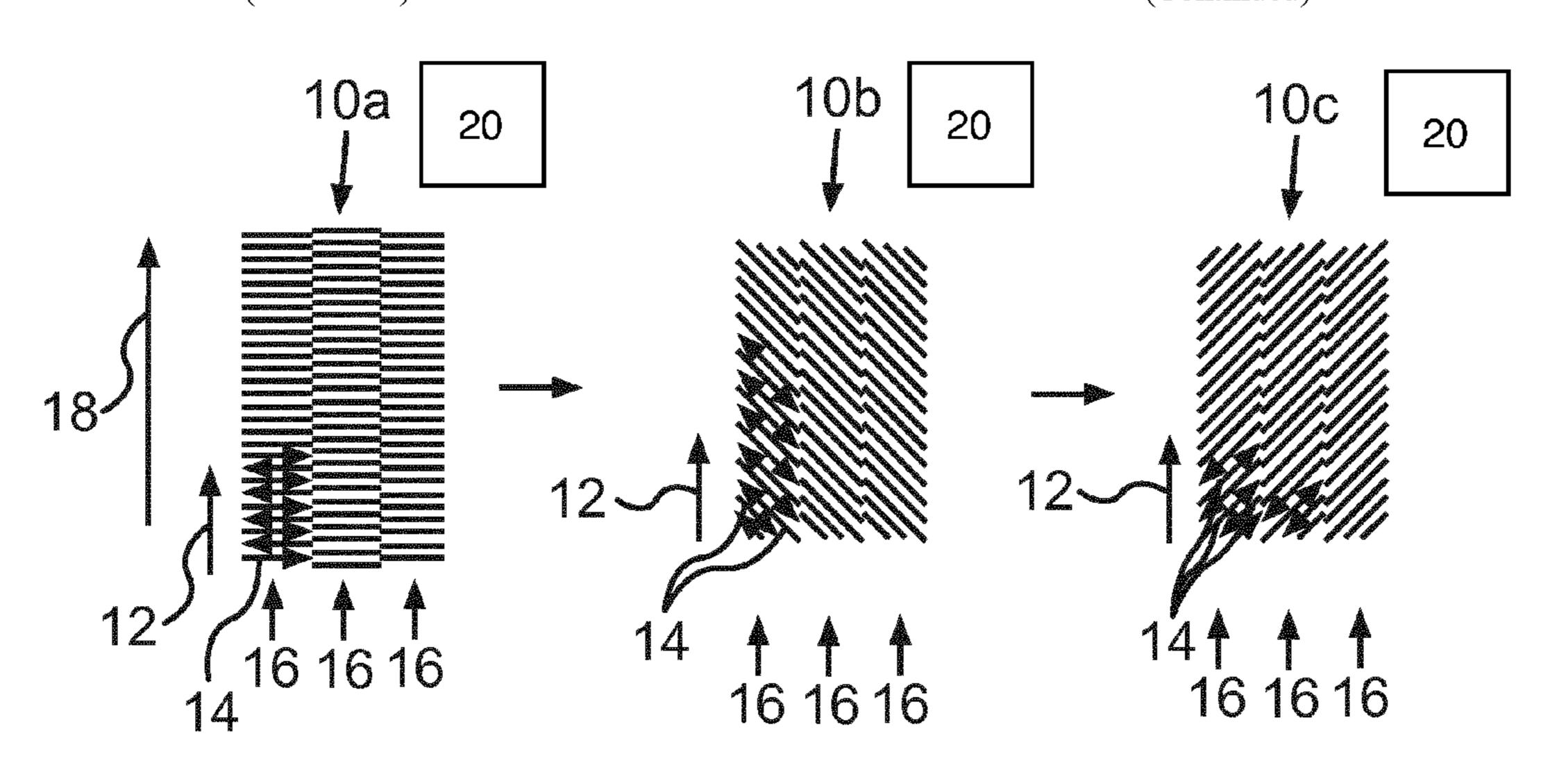
energy beam and the component platform are moved in relation to one another, in the form of a parallel arrangement arranged along a linear feed direction; lowering the component platform by a predetermined layer thickness in a lowering direction; and repeating the above-mentioned steps until the component region is completed.
