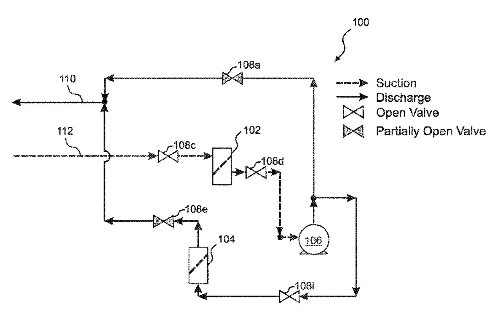
and solids into the environment is thereby avoided. Partially opened valves can be used to divert only part of the downstream flow for filter purging. Selectable paths can be included for which no filters are purged. The downstream flow can be divided and used to simultaneously purge a plurality of idle filters.
