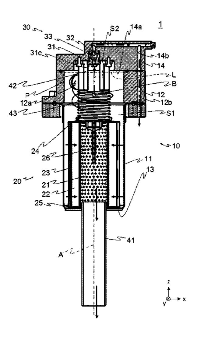
specific gravity than a liquid to be filtered. Thus, the float is pushed up by the liquid to occlude the first hole portion.
