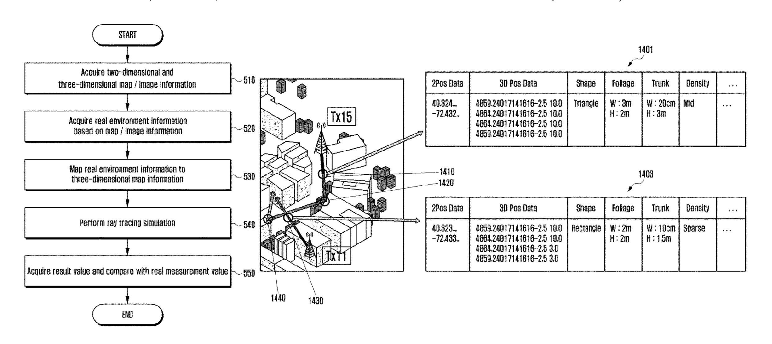
on the image information, determining property information of the at least one object, and analyzing communication environment for the area based on the property information. Signal attenuation occurs due to at least one of scattering, diffraction, or absorption of a signal by the at least one object.
