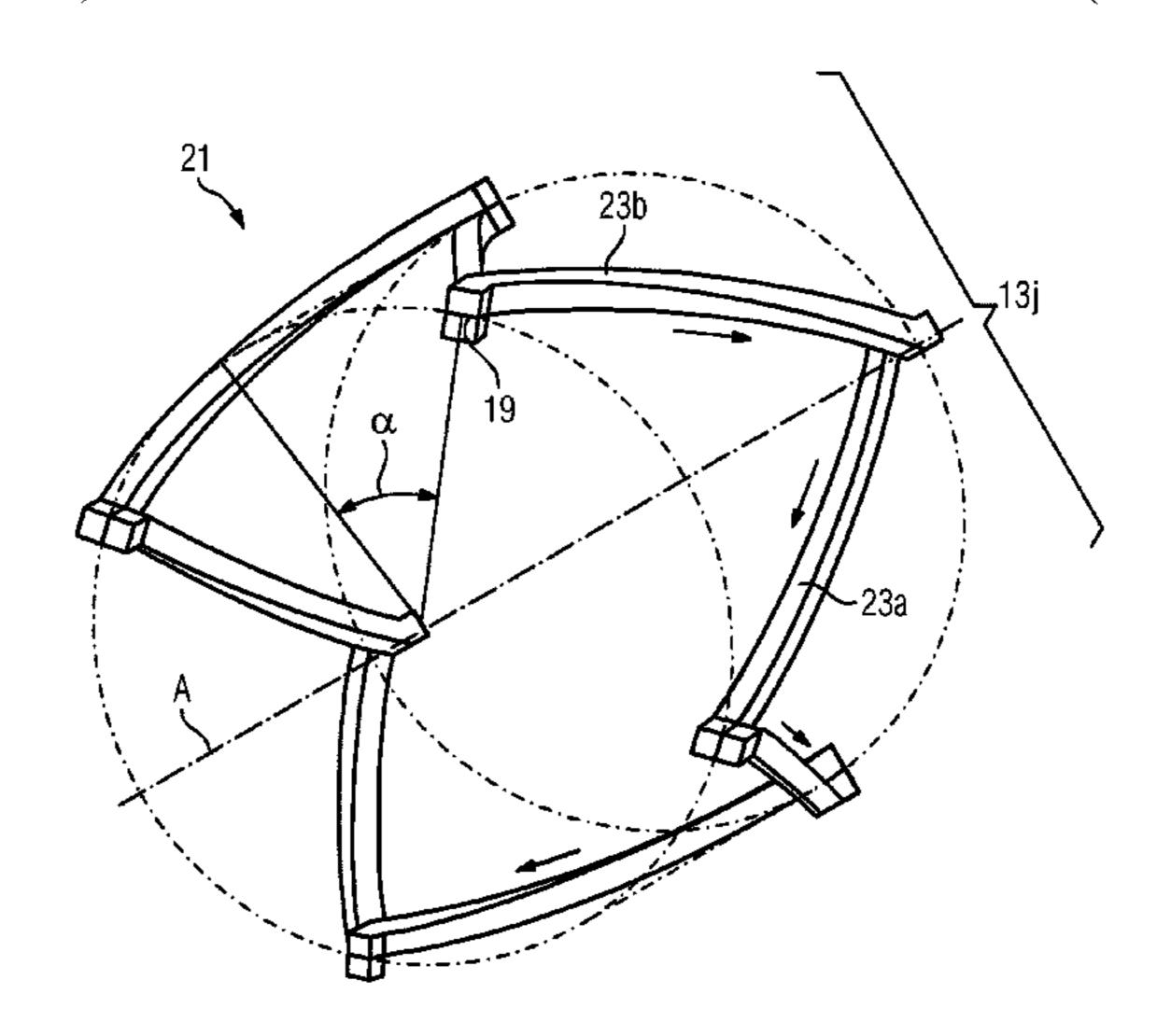
branch and the second conductor branch are arranged helically around the central axis over at least half of their respective lengths. The helically arranged conductor branches each have a pitch greater than a product of an axial length of the helical conductor branches and the number of magnetic poles.
