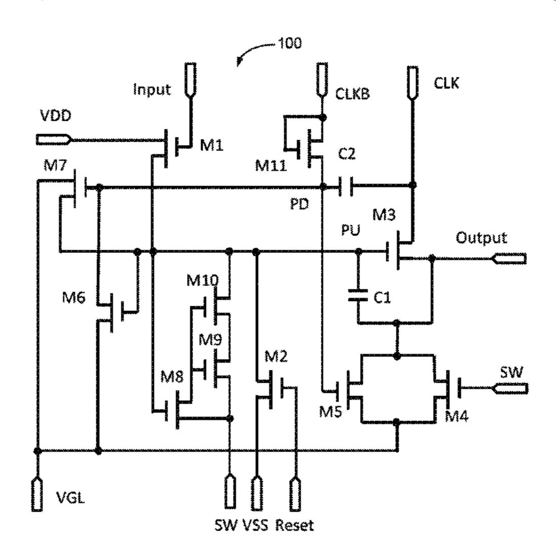
to switch back to the low voltage level after the touch scan stage to output the gate scanning signal without coupling interference of the touch scanning signal. The shift register circuit is compatible for driving either 60 Hz or high-frequency (>60 Hz) Full-in-cell touch sensing display panel.
