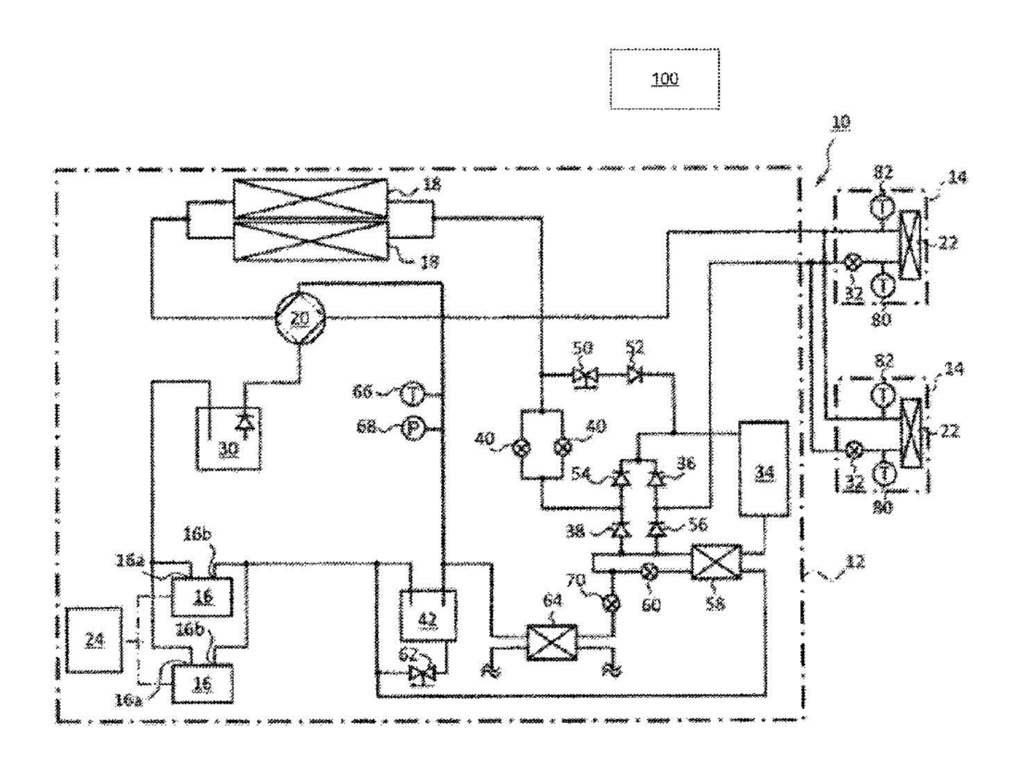
ture of the refrigerant flowing into the second heat exchanger and the temperature of the refrigerant flowing out from the second heat exchanger, and to control the opening of the flow rate adjustment valve based on the flow rate of the refrigerant to be supplied to the second heat exchanger.
