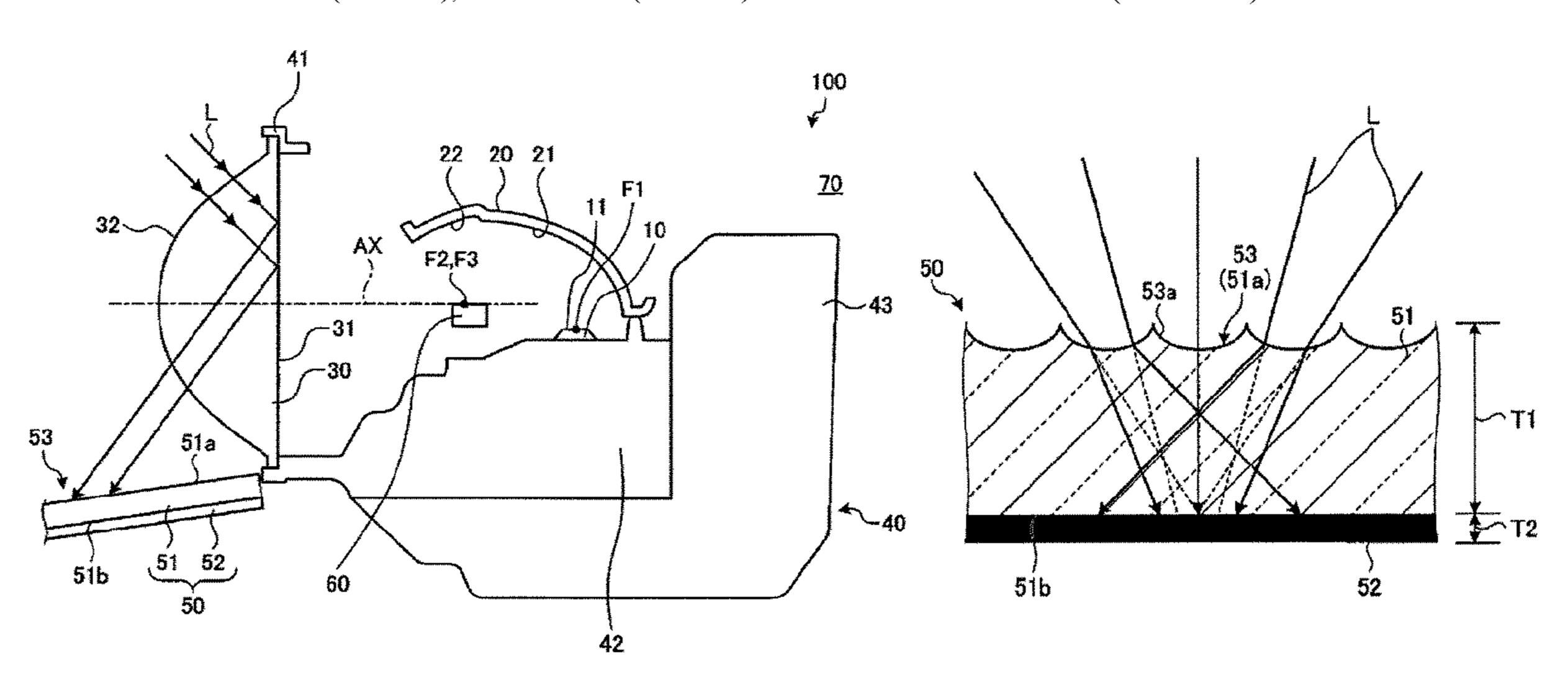
least in a portion of the light-transmitting member below the lens in the vehicle-mounted state.
