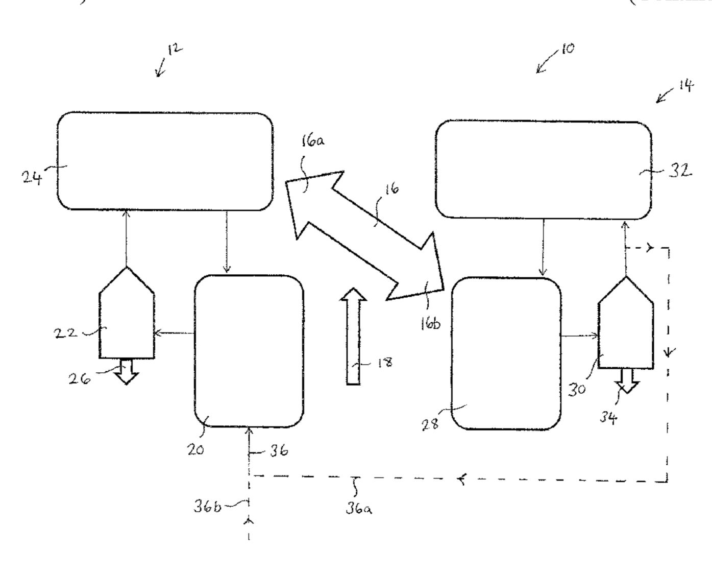
is stored as a pressurized vapor in a second storage vessel. In the discharge mode vaporized first phase change material is expanded by a first expander, or the vaporized second phase change material is expanded by a second expander.
