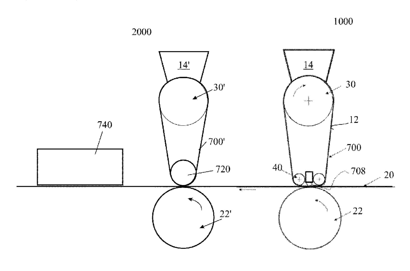
surface are pressed against each other to cause transfer to the surface of the substrate of the particles that have been rendered tacky.
