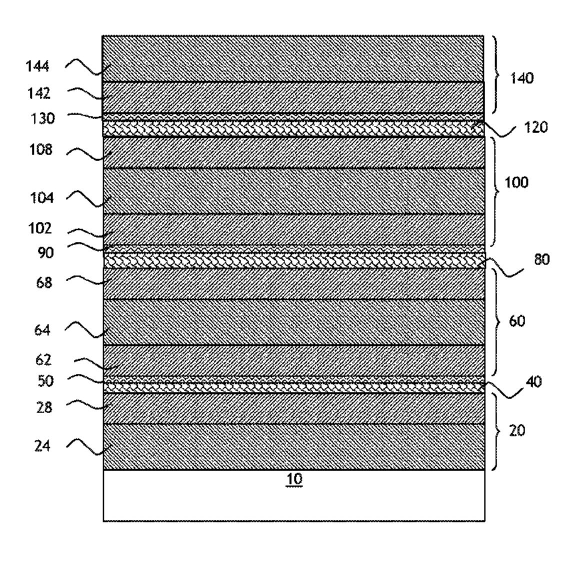
M1 and M2 each have an optical thickness Eo1 and Eo2 satisfying the following equation: Eo2<1.1 Eo1.
