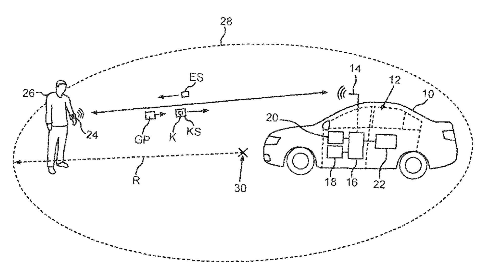
instantaneous geoposition (GP), the control device checks whether the emitted instantaneous geoposition (GP) is within a delimited, predetermined region, which is stored in the control device. The central locking system is finally unlocked when the emitted instantaneous geoposition (GP) is within the delimited, predetermined region.
