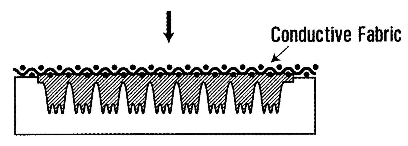
Stage 3. Laying a conductive fabric above silicone before curing
