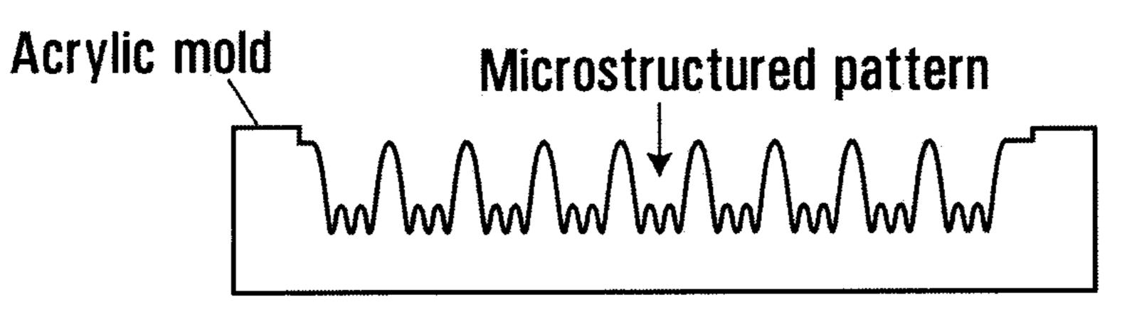
Stage 1. Development of microstructure mold with CO<sub>2</sub> Laser cutter
