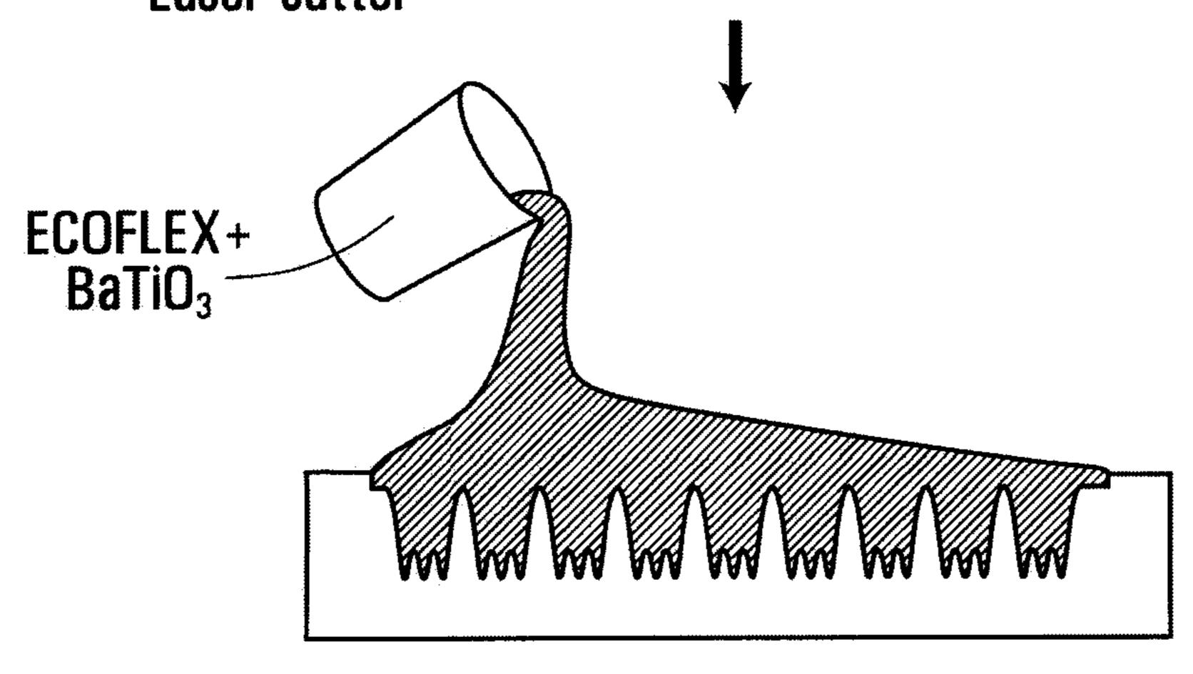
Stage 2. Spreading the mixture of ECOFLEX doped with nanoparticles of BaTiO<sub>3</sub> over mold
