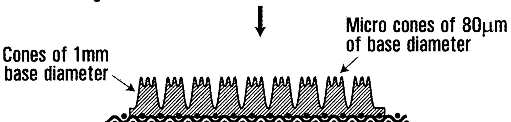
Stage 4. Microstructured ECOFLEX and  $BaTio_3$  silicone dielictric with conductive fabric
