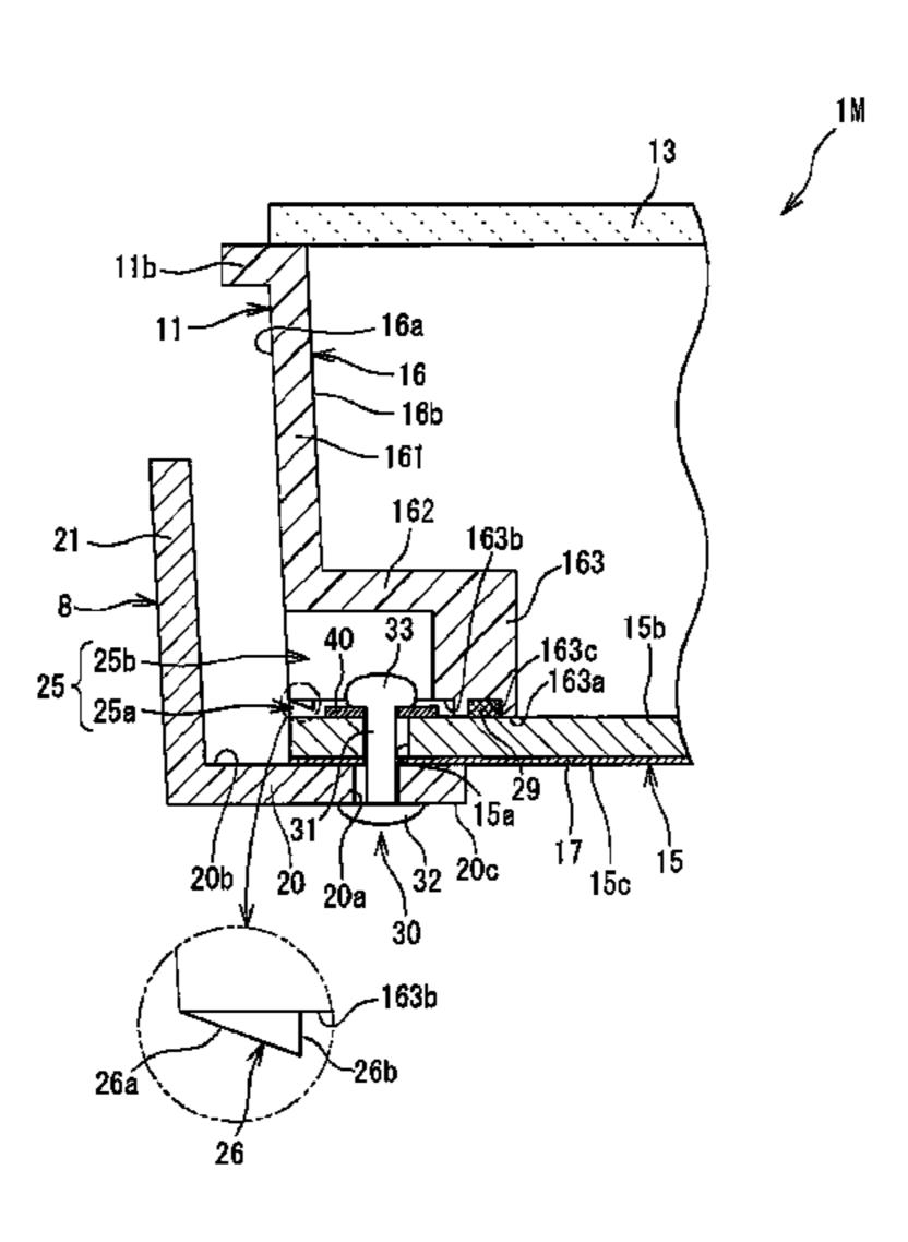
being configured to be passed through the support plate and the bottom plate to be inserted into the washer, the head formed at one end portion of the shank portion, the rivet being configured to sandwich and fasten the support plate and the bottom plate between the washer and the head by an other end portion of the shank portion being deformed so as to have an enlarged diameter.
