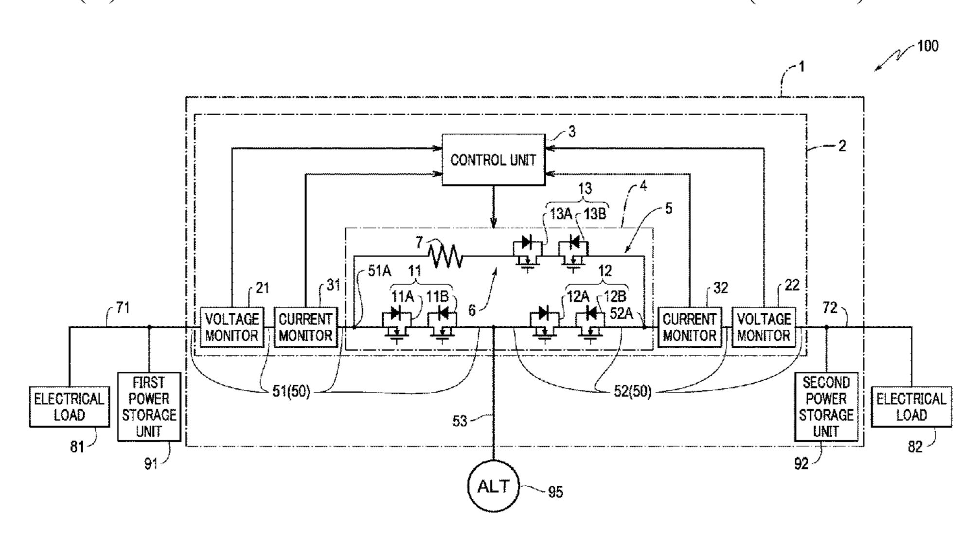
a series circuit in which a resistor and a third switch are connected in series to each other, the series circuit having one end electrically connected to a portion between the first switch and the first power storage device, and another end electrically connected to a portion between the second switch and the second power storage device; and a controller configured to turn the first switch, the second switch, and the third switch on/off.
