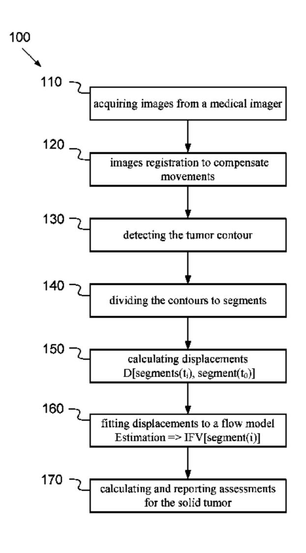
displacement to a flow model and extracting an estimation of the interstitial fluid velocity. The estimated interstitial fluid velocity of the segments provide characterization of the solid tumor and includes an assessment of the tumor interstitial fluid pressure, the tumor drug delivery efficiency, and the tumor prognostic or metastasis risk.
