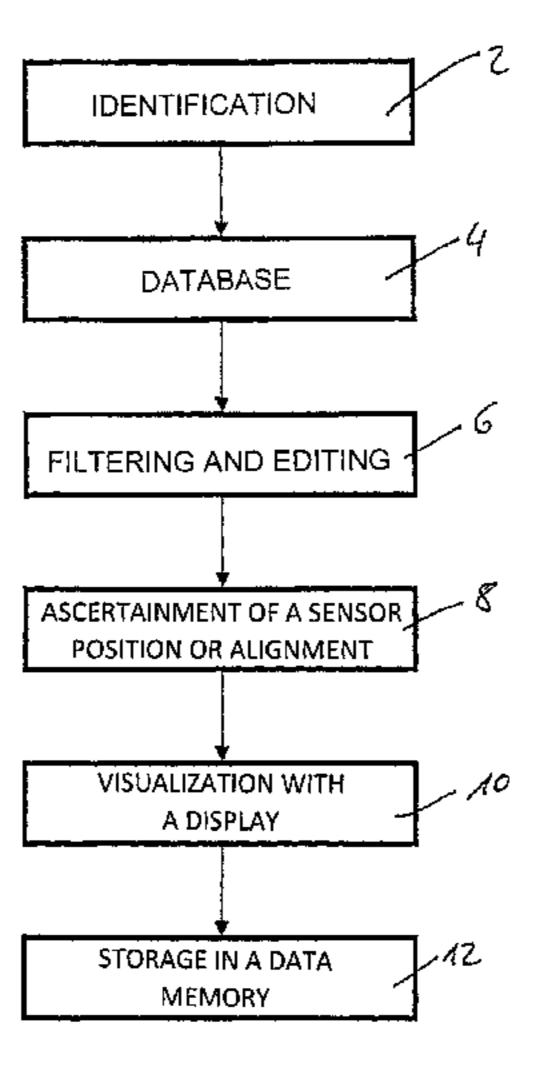
the user with the aid of the provided data and specified sensor characteristics an intended position and/or intended alignment of a sensor can be visualized and stored for later use during installation.
