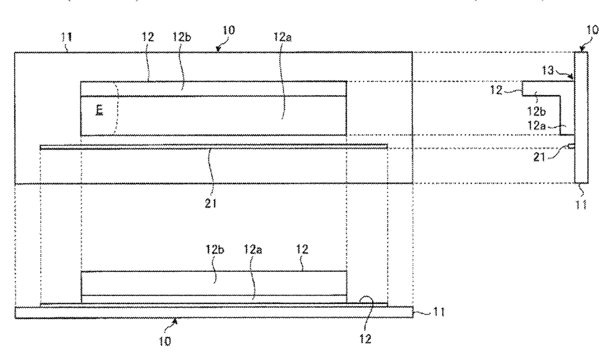
when a load is applied to the adherend in a reference state in which debonding of the adhering portion does not occur. The debonding detecting method includes: applying a load to the adherend; measuring a strain of the adherend by the optical fiber sensor; and the determining presence or absence of debonding based on comparison result obtained by comparing measured strain data measured in the measuring and the reference strain data.
