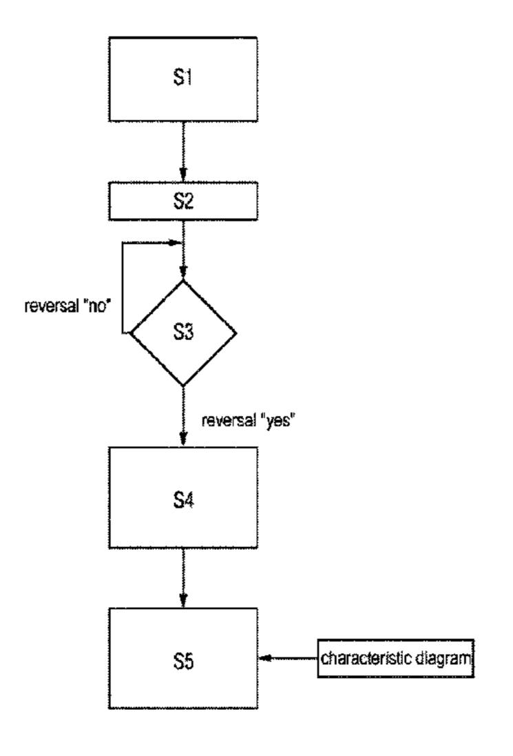
the rotational speed gradient in such a way that the influence of the reversal of the direction of rotation on the position of the camshaft is compensated.
