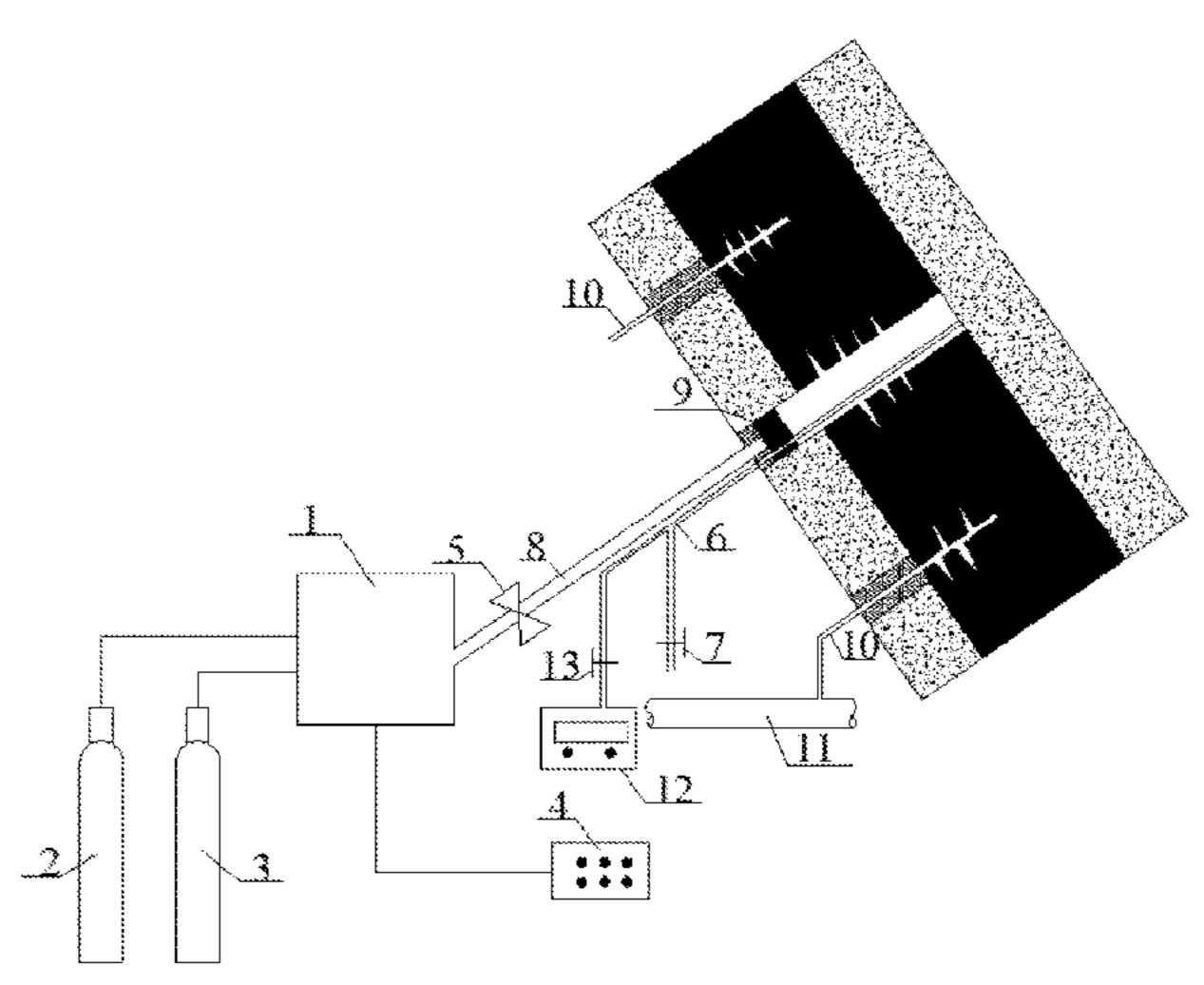
temperature and high-pressure impact wave. High-temperature vapour is injected into the drill holes by the heat injection and gas injection extracting pipe to promote desorption of the coal masses.
