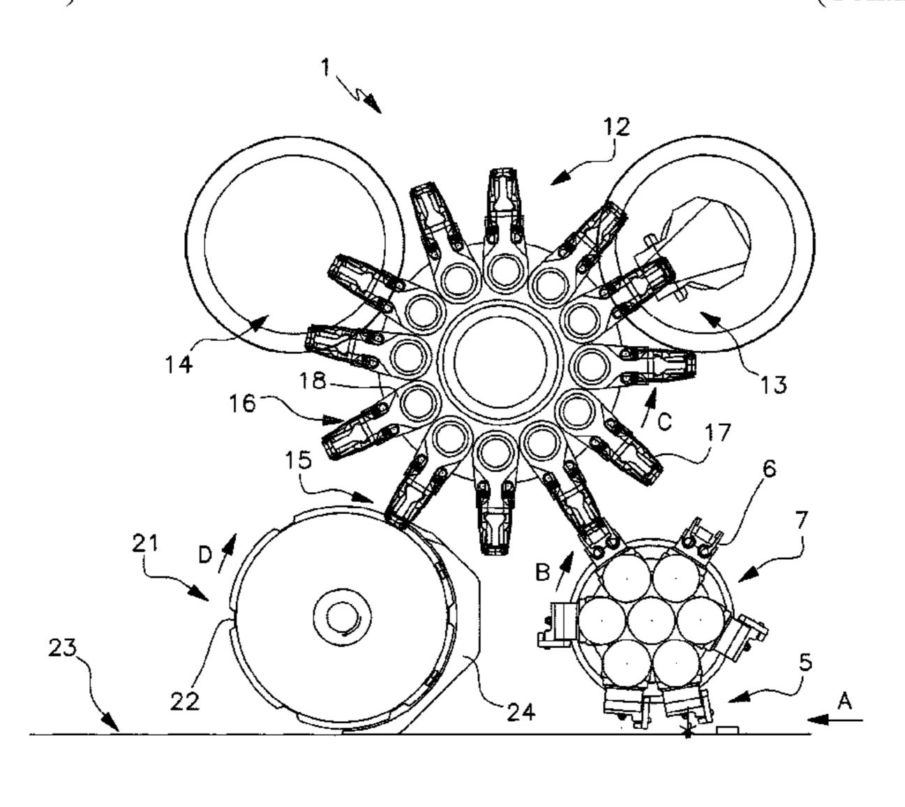
lows folded ends of the wrapping is performed to obtain the airtight closure of the package.
