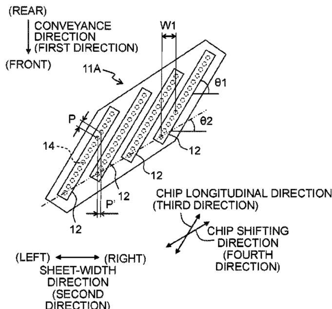
fourth nozzle chips included in the head units partially overlap with each other in the first direction.
