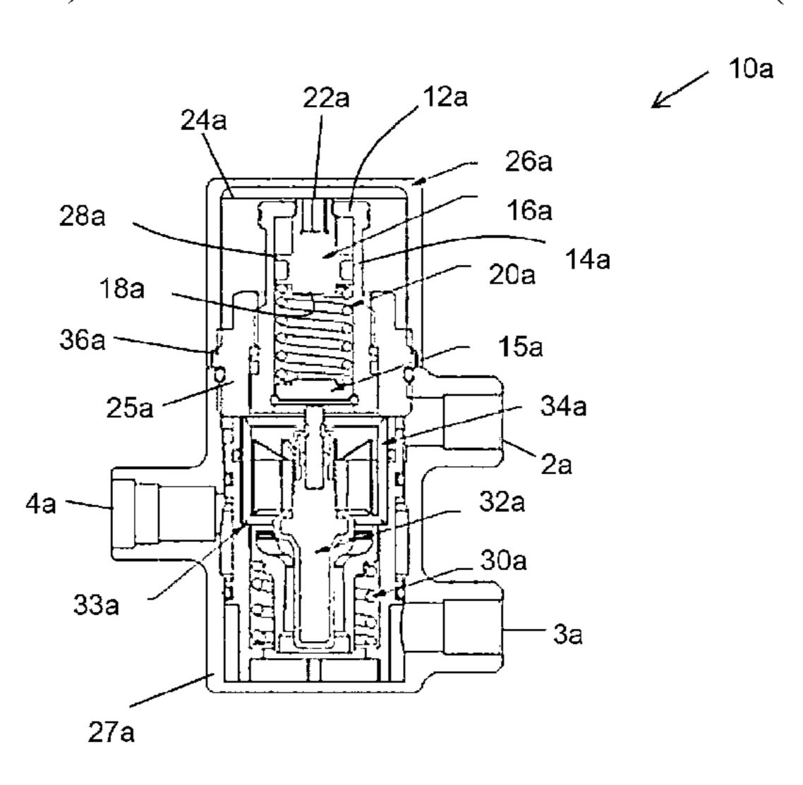
during movement thereof; and a plunger extending into the housing, the plunger configured to engage the overtravel spring, wherein rotating the plunger adjusts the resistance applied onto the thermostatic element from the overtravel spring.
