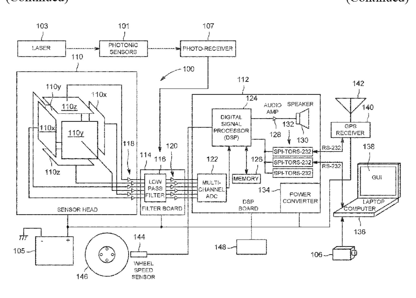
pertaining to hazardous energy to locate an energized object proximate a street; and an indicator, coupled to the processor, that alerts a user to a presence of the energized object in the electric field proximate the street.
